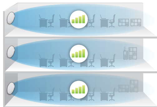
Pattern for wall-mount (H-plane, side view)
