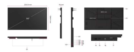
1. Speaker 2. Control Panel 3. OPS Slot 4. USB 2.0 5. RS-232 6. USB 3.0 7. USB-C 8. HDMI 1(ARC) 9. HDMI 2 10. HDMI OUT 11. HDMI 3 12. WiFi Slot 13. VESA® Wall Mount (800x600mm) 14. AC IN
