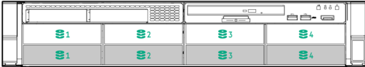
8LFF chassis with Universal media bay and optional 2SFF and optical drive shown
