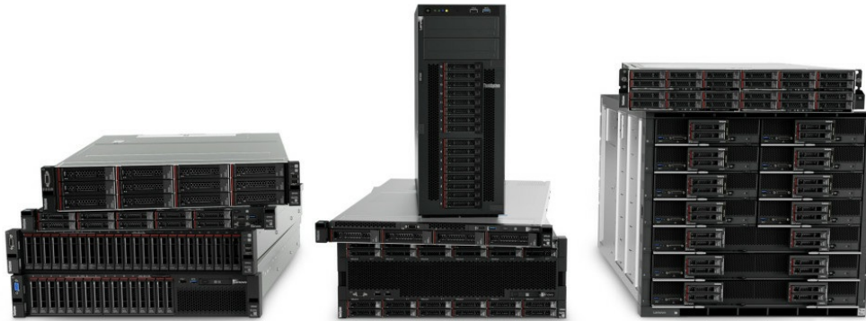
Figure 1. ThinkSystem servers include the XClarity Controller integrated service processor
